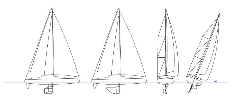
**Advantages**: allows the combination of good sailing performance and a low draft for accessibility to ports and mooring areas.
