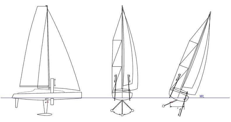
Advantage: considerably increases the righting torque (Cr) at current heeling angles (0 to 30 °) by moving the Cg sideways.
