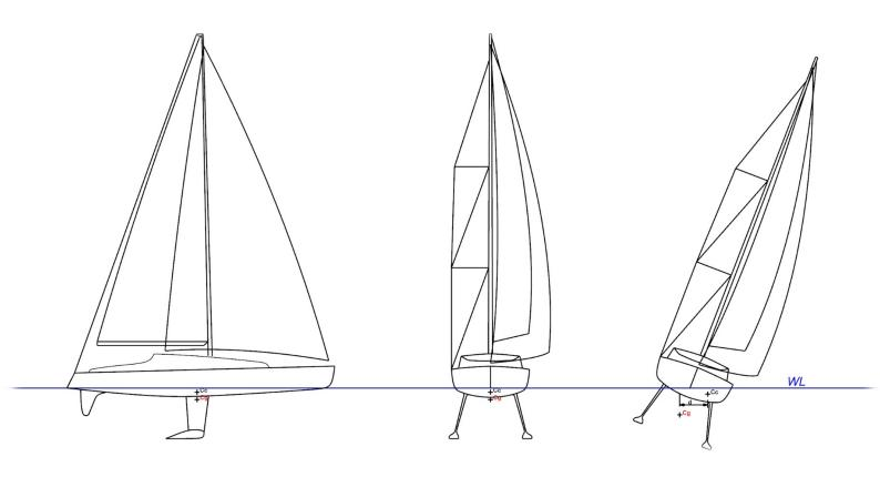
**Advantages:** same efficiency, easy handling, reliability, economy as for the single keel, with the added advantage of losing little anti-drift surface with the increase in heel and being able to land on both keels.
