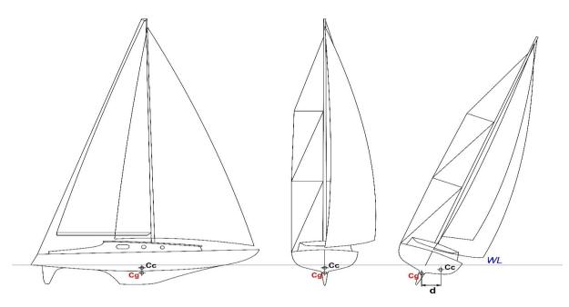
To increase the righting torque (Cr), without increasing the displacement (weight), it is therefore necessary to increase the horizontal distance (d) between the center of the hull (Cc) and the center of gravity (Cg) of the sailboat.
