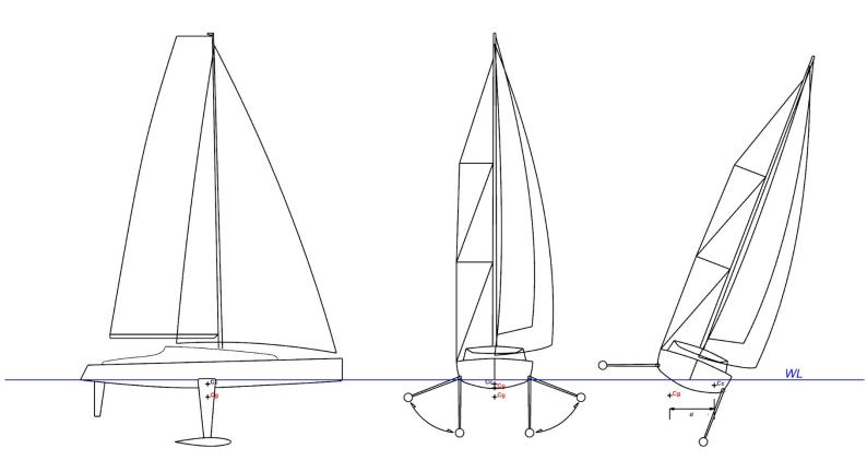
**Advantages:** partly combines the high righting torque (Cr) obtained by the tilting keel and the possibility of reducing the draft. Simpler maneuvers, two mobile appendages (electronically assisted) instead of three (no daggerboards necessary).
