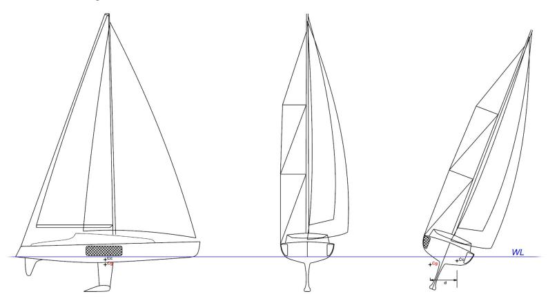
**Advantage:** increases the righting torque at current heel angles (from 0 to 30 °) by moving the Cg sideways.
